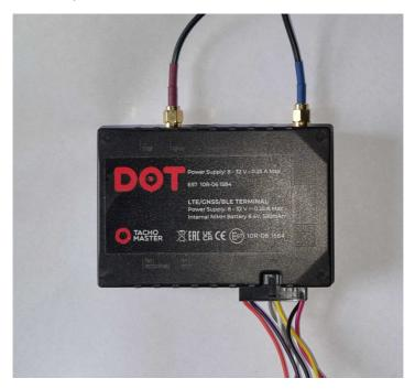
Please ensure that the GPS antenna has a clear sky view and has the black plastic side facing the sky. The GSM antenna must not be attached to metal to ensure a better signal.
