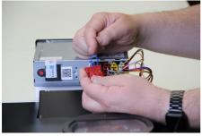
If you removed a Red 'C' Connector, check to see if there is a link wire fitted pin 7 to 8.
