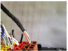
There was no link wire on the original red plug so the black loop was cut on the DOT red plug for consistency. However the impedance was still low, indicating an additional resistance loop.
